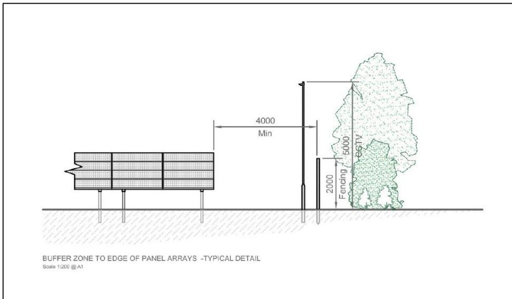
The solar panels will be spaced to avoid shadow and set on a frame supported by stakes. There will be minimal disturbance to the ground, the units will also be sited to achieve optimum exposure for solar energy absorption. This construction method allows the scheme to be easily reversed in the future, simply by pulling out the framework. There would be no foundations used.
